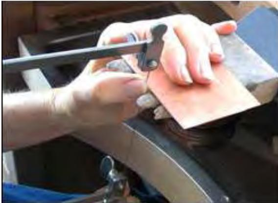
**STEP 1:** Cut metal sheet with saw blade or shape cutter
