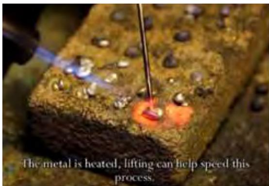
**STEP 1:** Heat the plain metal and place a solder alloy piece on top of it
