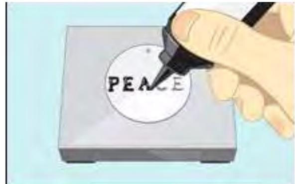
**STEP 4:** Remove tape, wipe area clean, apply enamel or permanent colouring to the etched stamp
