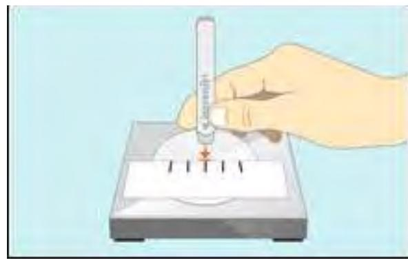
**STEP 2:** Place stamp on metal and move towards the tape without scratching the metal
