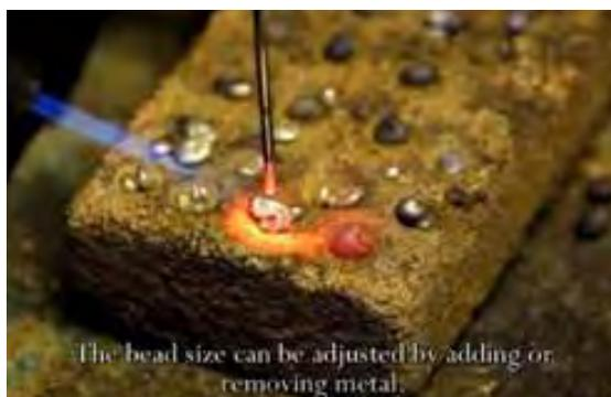
**STEP 3:** Adjust bead size by adding or removing metal when molten
