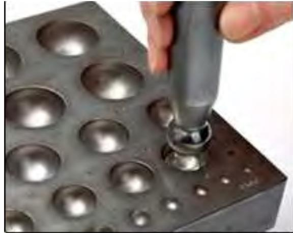
**STEP 2:** Put in a smaller dent and keep hammering lightly
