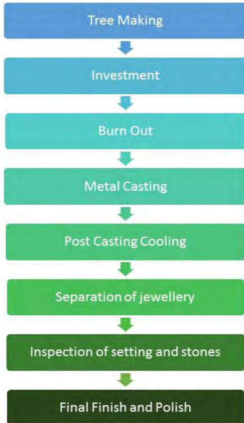
Fig. 2.2.3.1: Post Wax Setting Process
