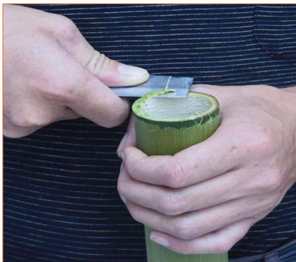
● Figure 2.2.1 - STEP 2: Flatten the edges of culm
