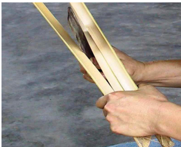
● Figure 2.2.1 - STEP 4: Separate the slivers
