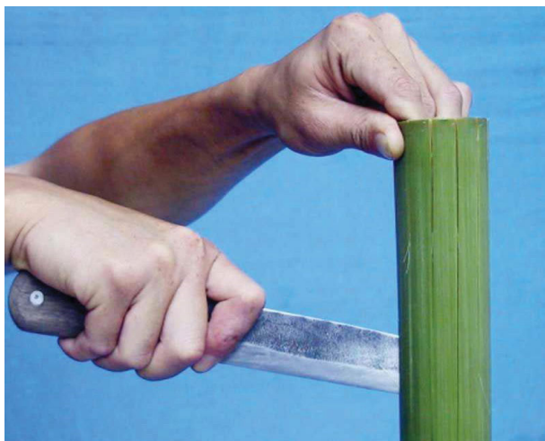
● Figure 2.2.1 - STEP 3: Divide the culm into slivers of equal width
