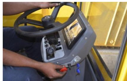
Fig no. 1.4.6.c : Parking Brake Switch
