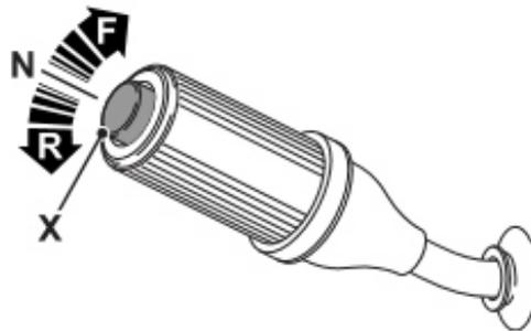
Fig 1.4.3.2.1 Transmission Lever
