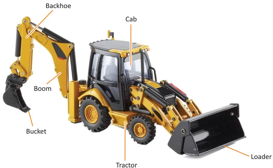
*Fig 1.4.2 Backhoe Loader Parts*
