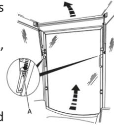
**Note:** When closing the window, make sure that the window wiper lead does not get trapped
