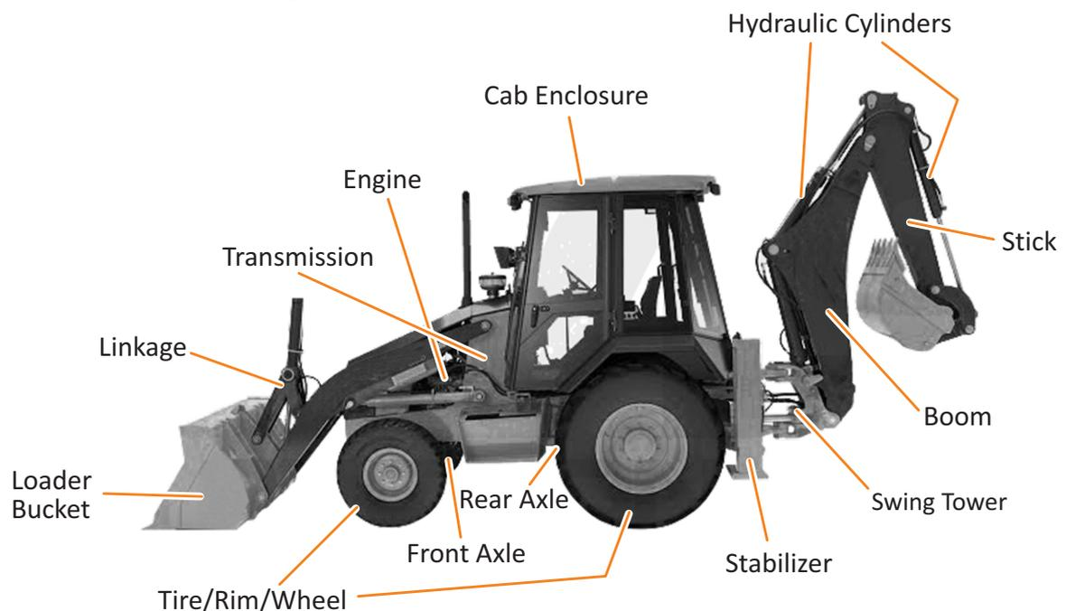
Fig 1.4.2.1 General Backhoe Loader Specifications
