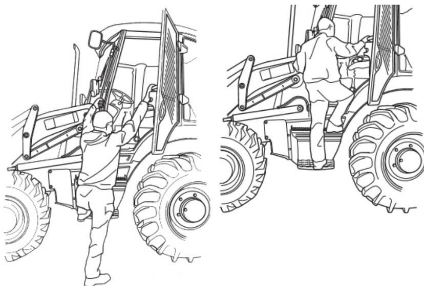
Fig. No. 2.3.1 Entering and Exiting the Backhoe Cabin
