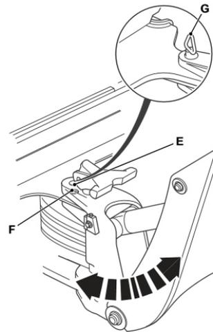
E Hole (in the kingpost), F Hole (in the mainframe)
