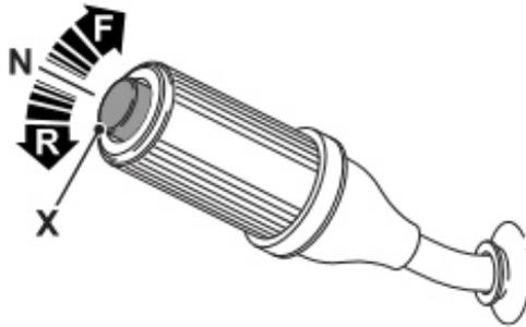
Fig 1.4.3.2.1 Transmission Lever
