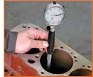
**Fig 4.4.9:** Calculating diameter using bore gauge
