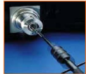
*Fig 8.3.2: Removing bearing from housing*
