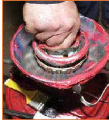
**Fig 7.2.2:** Apply grease on bearing
