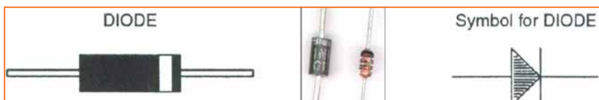
Fig 5.1.2: Diode and its symbol
