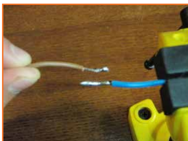
Fig 6.2.6: Soldering of two wires
