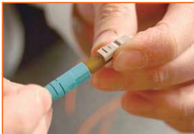
Fig 6.2.7: Completion of fiber optic cable termination
