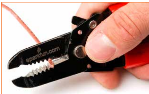
Fig 6.2.2: Wire stripping
