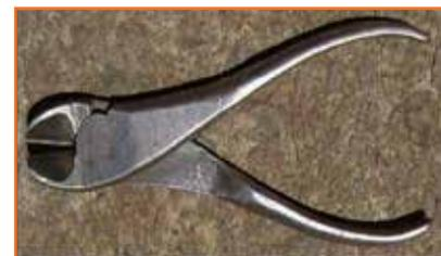
*Fig 5.2.5: Side cutting plier*
