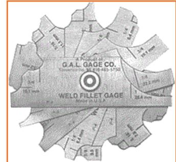
Fig 7.2.11: Fillet weld gauge
