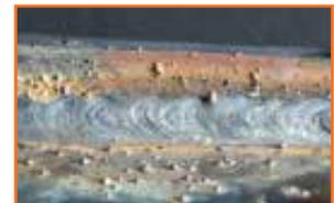
*Fig. 7.1.1: Weld spatter*
