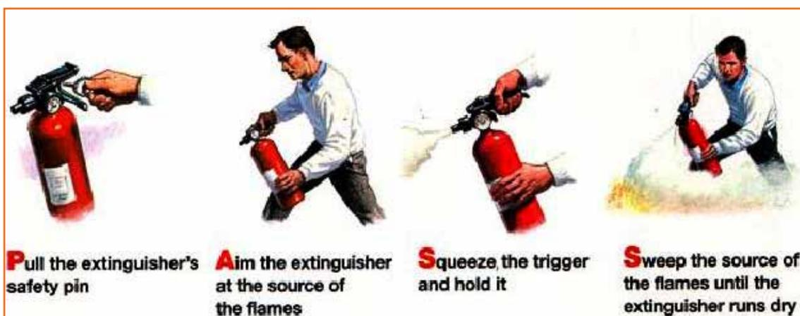
Fig 2.5.2: Using fire extinguisher
