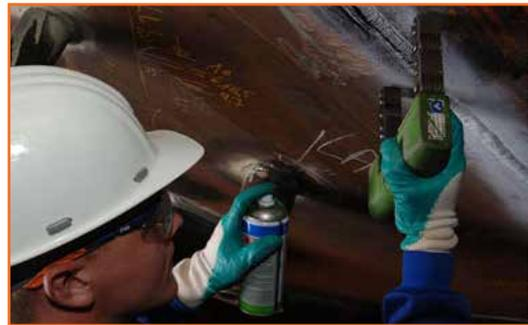
Fig 7.2.8: Magnetic Particle Inspection
