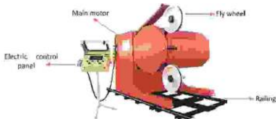
Fig. 2.1.3. Parts of a Wire saw machine
