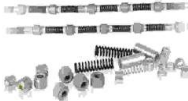
Fig. 2.1.10. Parts of a diamond chain
