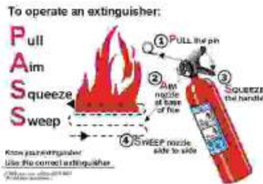
Fig. 5.4.5. Procedure for using Fire Extinguisher
