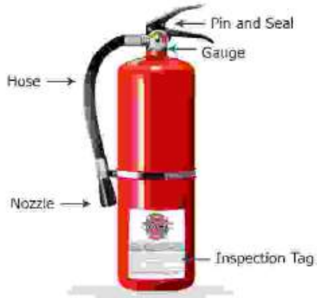
Fig. 5.4.4. Parts of Fire Extinguisher
