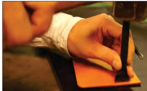
**STEP 4:** Strike pronging chisel with rawhide mallet
