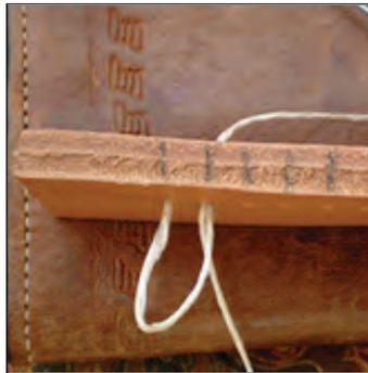
**STEP 9:** Insert the lower needle/ thread from the bottom **ALONGSIDE** the thread filling the hole. Take care to insert the needle **ALONGSIDE** the thread, do not **PIERCE** it!
