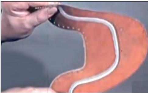
**STEP 5:** Check the edges of the upper are shaved, to prevent thickness where they overlap or fold
