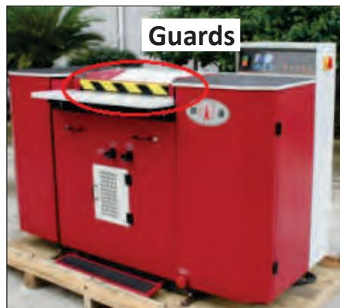
Fig 6.2.3 Splitting machine Guards
