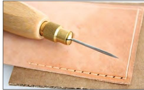
**STEP 8:** Use 1 prong punch or scratch awl to end or fill in spaces, or to free form pattern
