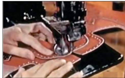
**STEP 6:** Stitch the tip to the Vamp using flat bed machine and join quarter with the vamp using post bed machine as specified in the job card
