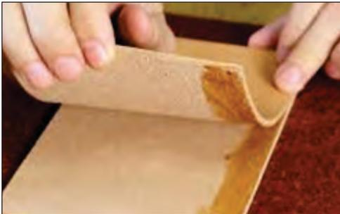
**STEP 1:** Fix pieces together with glue before punching holes for stitching
