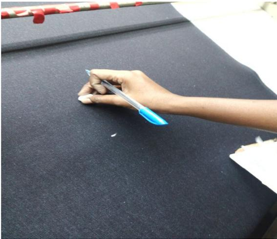
*Fig 3.3.4: Marking fabric faults*
