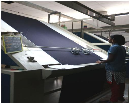
Fig. 2.2.2: Proper illumination in the inspection Table
