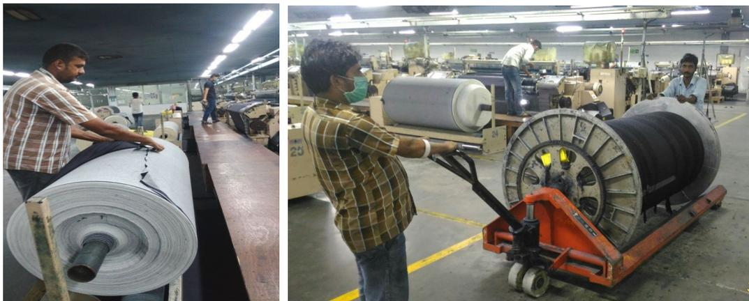
Fig 3.2.4: Material handling of doffed rolls
