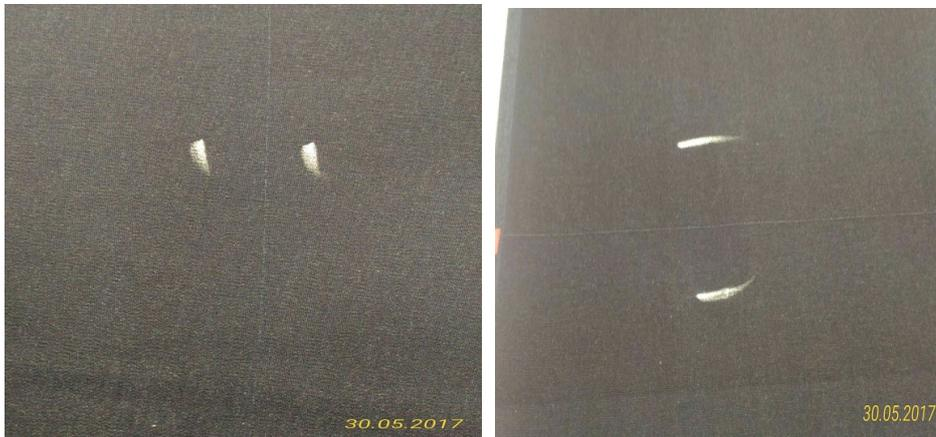
*Fig 3.1.4: Warp direction and weft direction fault*
