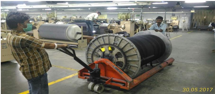
*Fig 4.1.1: Trolley truck to transport the load*
