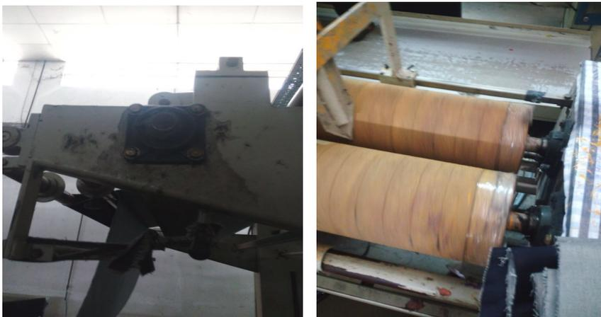
*Fig 4.1.2: Greasing points to be maintained regularly*
