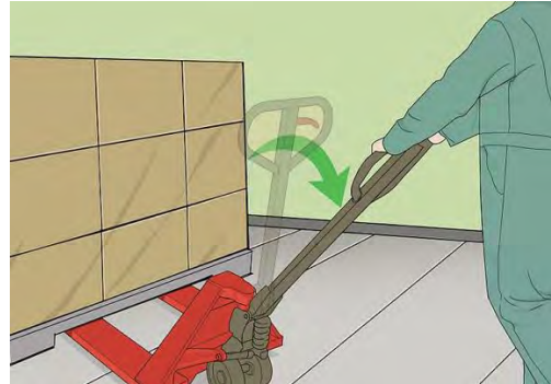
Step 4: Use the handle to jack up the pallet
