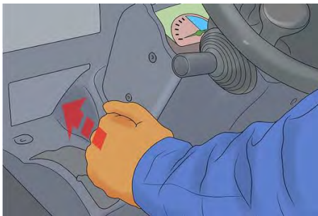
Step 5: Use shifter to change the direction
