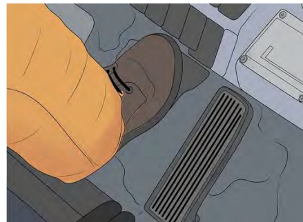
Step 4: Depress the brake pedal before releasing emergency break.
