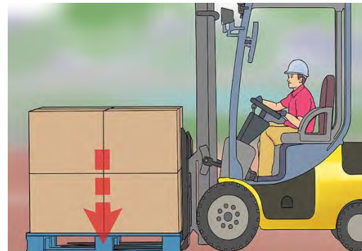
Step 16: Lower the forks until pallet is set
