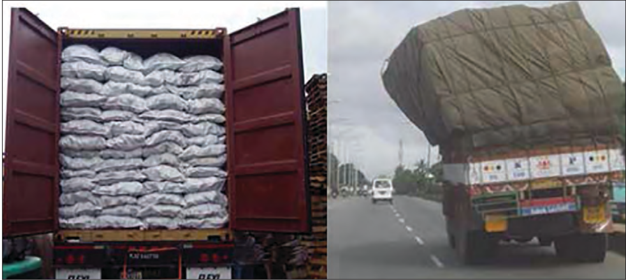
Fig 6.6- Correct way and wrong way of loading
