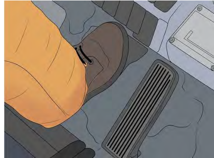
Step 4: Depress the break pedal before releasing emergency break.
