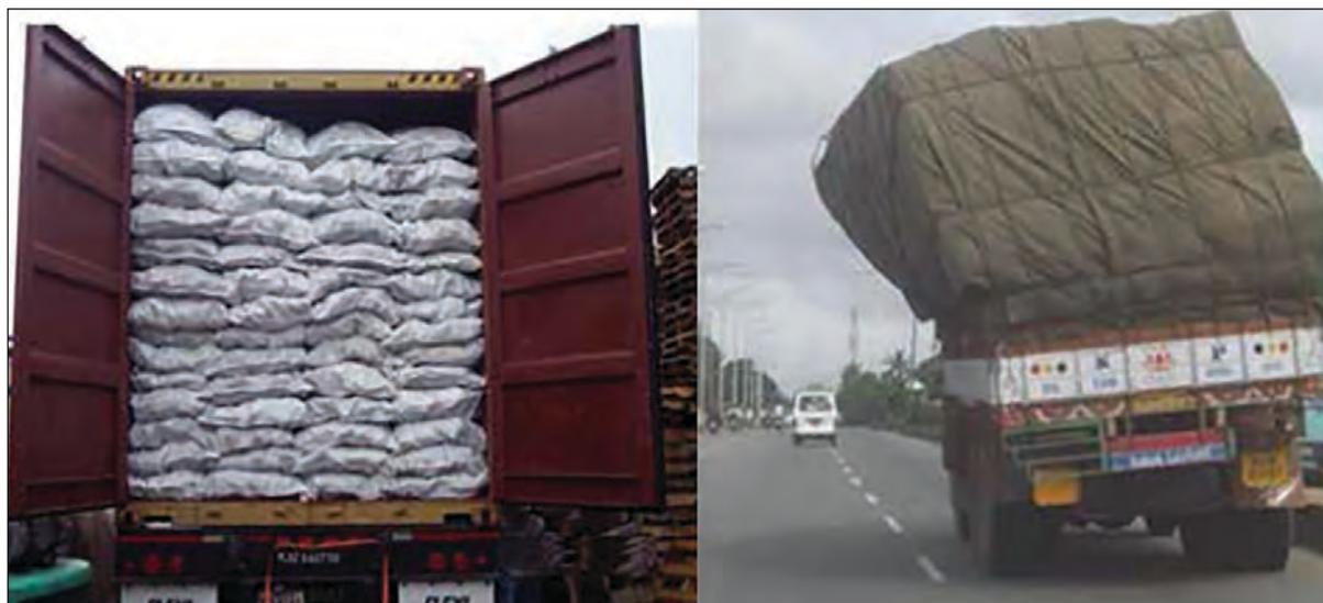
Fig 6.6- Correct way and wrong way of loading
