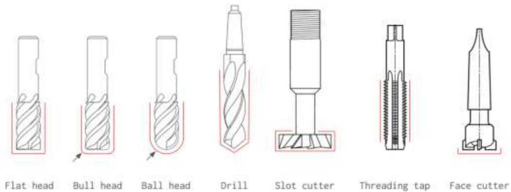
Fig 4.3.1 Types of cutting tools
