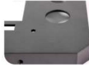
**Powder coating** adds a wear and corrosion finish to the surface of the parts. Has higher impact resistance compared to anodizing. Large range of colors available. Can be applied to any metal
