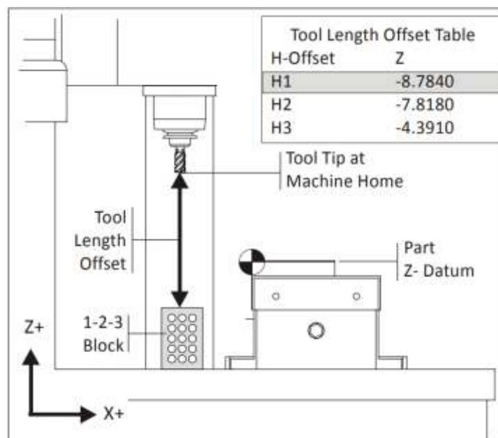
Fig 5.2.1 Setting tool length Offsets
