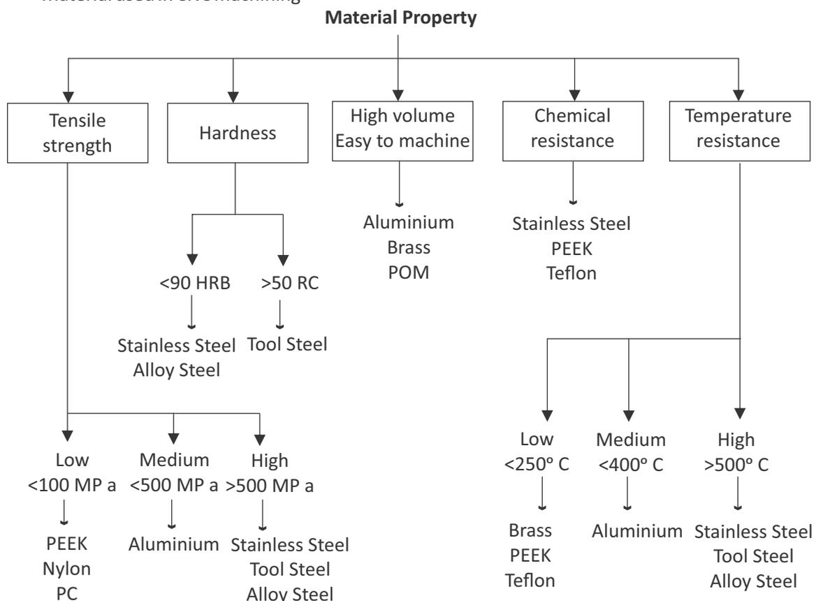
Fig 4.4.1 Material used in CNC machining
