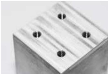
As **Machined** parts have minor visible tool marks. The standard as machined surface roughness (Ra) is  $3.2 \mu\text{m}$ . Surface finish requirements can be increased to 1.6, 0.8 and  $0.4 \mu\text{m}$ .
