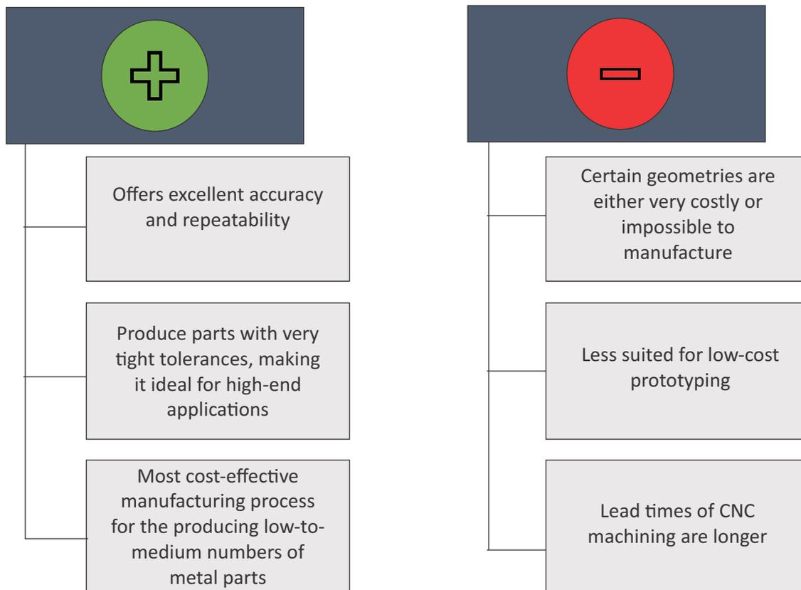
Fig 4.10.1 Potential benefits and limitations of using CNC machine
