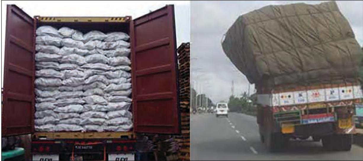
Fig 6.2.1- Correct way and wrong way of loading
