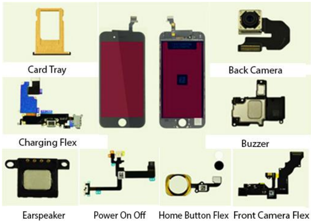
Fig 1.5.1: Basic parts of a mobile phone
