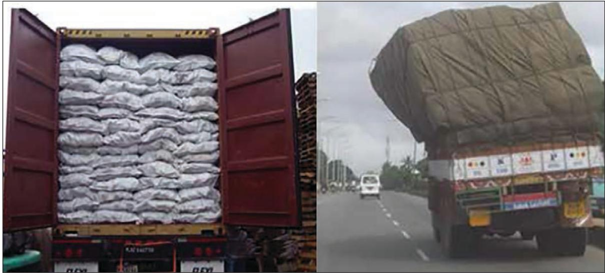
Fig 5.2.1- Correct way and wrong way of loading
