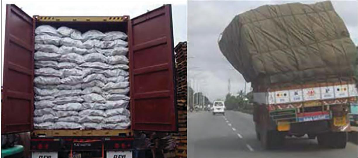
Fig no. 6.1.12 - Correct way and wrong way of loading
