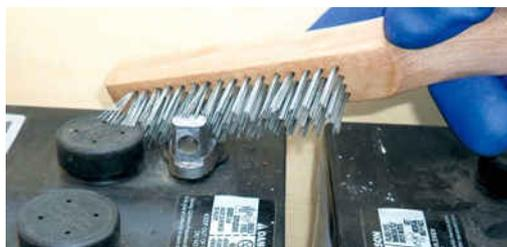
Fig. 2.5.13 Cleaning of Batteries
