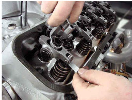
Fig. 3.4.3 Adjusting Tappet Clearance
