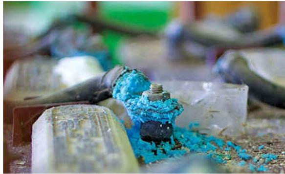
Fig. 2.5.14 Corrosion on the Battery Terminals
