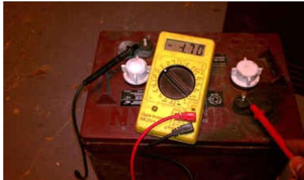
Fig. 2.5.9 Checking Battery Voltage
