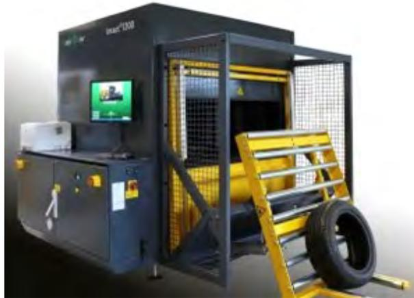
Fig. 2.1.7. Shearography tyre test machine
