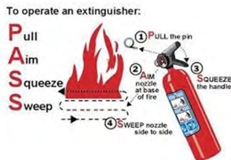
Fig. 9.4.10. Method of operating Fire extinguisher
