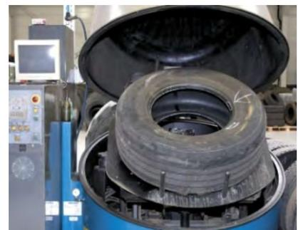
Fig. 9.1.7. Retreaded tyre curing
