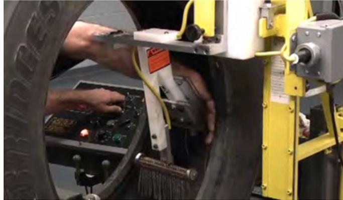
*Fig. 2.1.6. Electric sparks tyre inspections machine*
