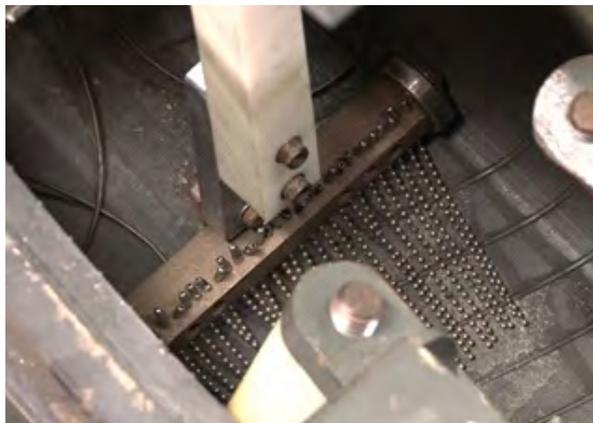
Fig. 3.2.4 Tyre electric spark inspection process
