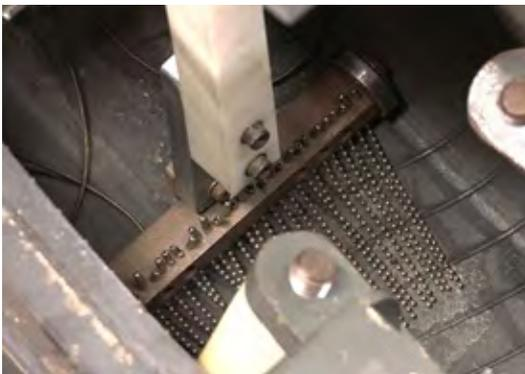
*Fig. 2.1.6.-1 Electric sparks tyre inspections machine*
