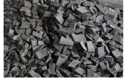
Fig. 4.2.6. Shredded tyre for recycling
