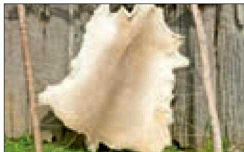
**STEP 11(d):** Assist in clipping the hides by tying across all the edges of the leather to the wooden frame.
