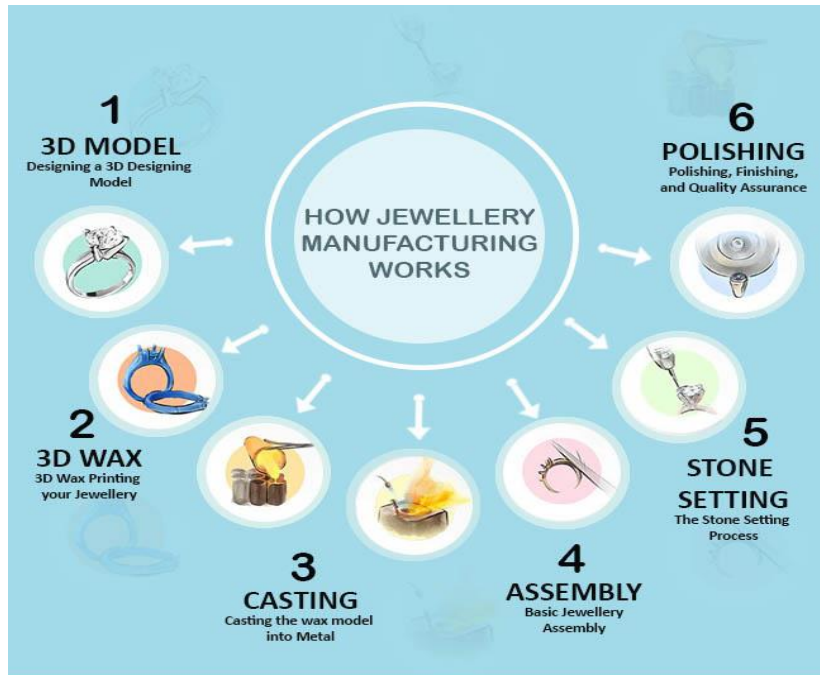
Fig. 1.1.3: Casting jewellery manufacturing process
