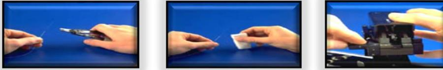
Fig 2.3.8: Cleave the fibre
