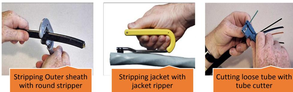
Fig. 2.3.7: Splicing preparation
