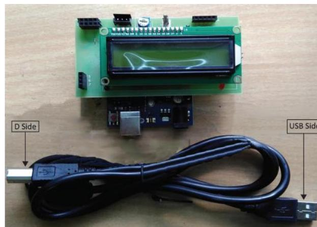
Fig 4.3.3: Connect cable to the Arduino board
