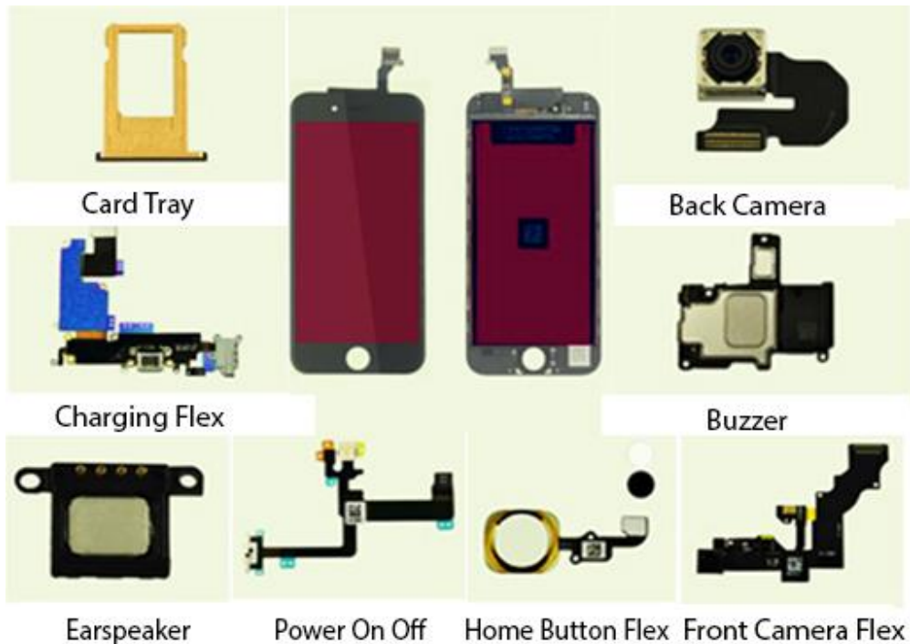
Fig 1.5.1: Basic parts of a mobile phone
