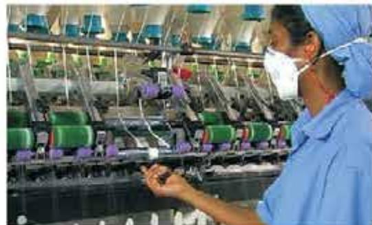
*Fig 5.1.10: Cleaning lapping using index finger*
