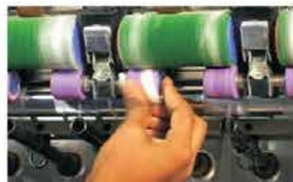
Fig 4.3.2: Clean roller lapping waste
