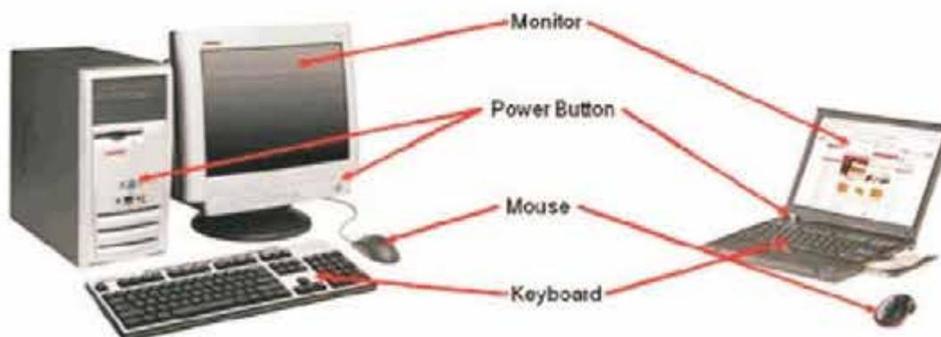
Fig 10.2.1: Basic parts of computer
