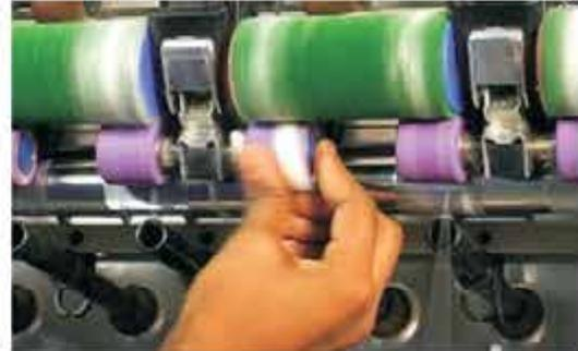
*Fig 5.1.8: Clean lapping using thumb finger*
