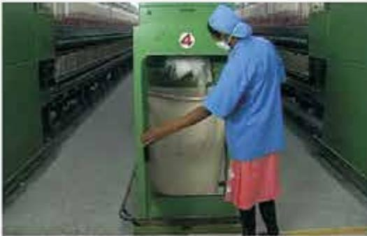
*Fig 5.1.5: Open the door at m/c off end*
