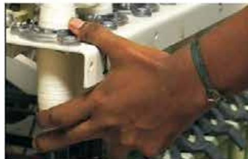
**STEP 4:** Hold spindle firmly by index & middle finger and place thumb on ring
