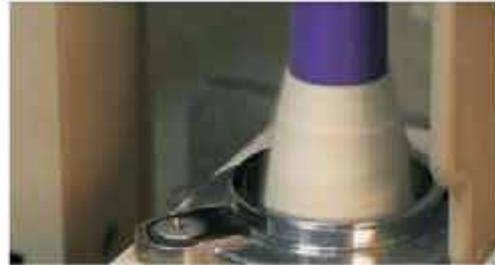
Fig 4.1.5: Traveler fly (No traveller found in ring)
