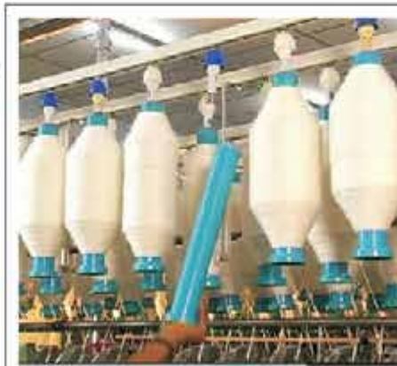
Fig 3.1.1: Remove empty bobbin
