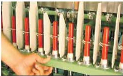
**STEP 7:** Release left hand from spindle
