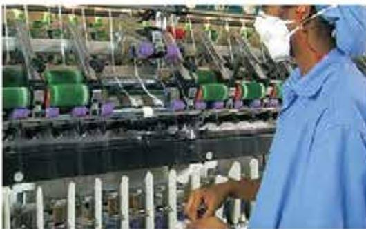
*Fig 5.1.9: Bottom roller lapping*
