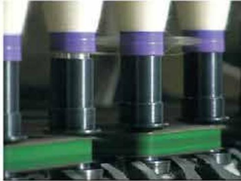
Fig 4.4.1: Improper seating of cop in the spindle
