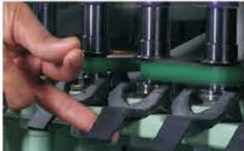
**STEP 1:** Apply brake using middle finger
