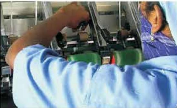
**STEP 3:** Pass end in roving condenser guide.
