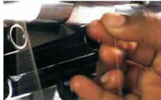
**STEP 2:** Join the end with the drafted material & twist the yarn slightly
