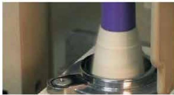
*Fig 4.1.2: Traveler fly (No traveller found in ring)*
