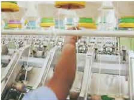
**STEP 1:** Cut running roving & wrap around guide rod
