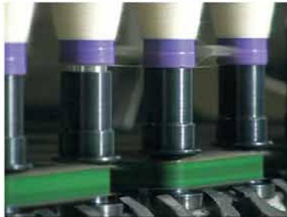
*Fig 4.2.1: Improper seating of cop on spindle*
