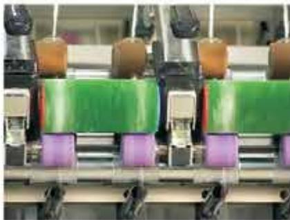
Fig 4.4.2: Material passage at drafting zone
