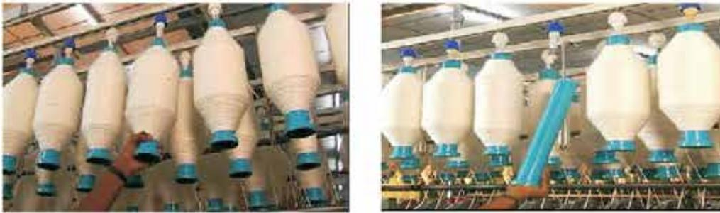
*Fig 6.1.1: Handling method of roving bobbin*
